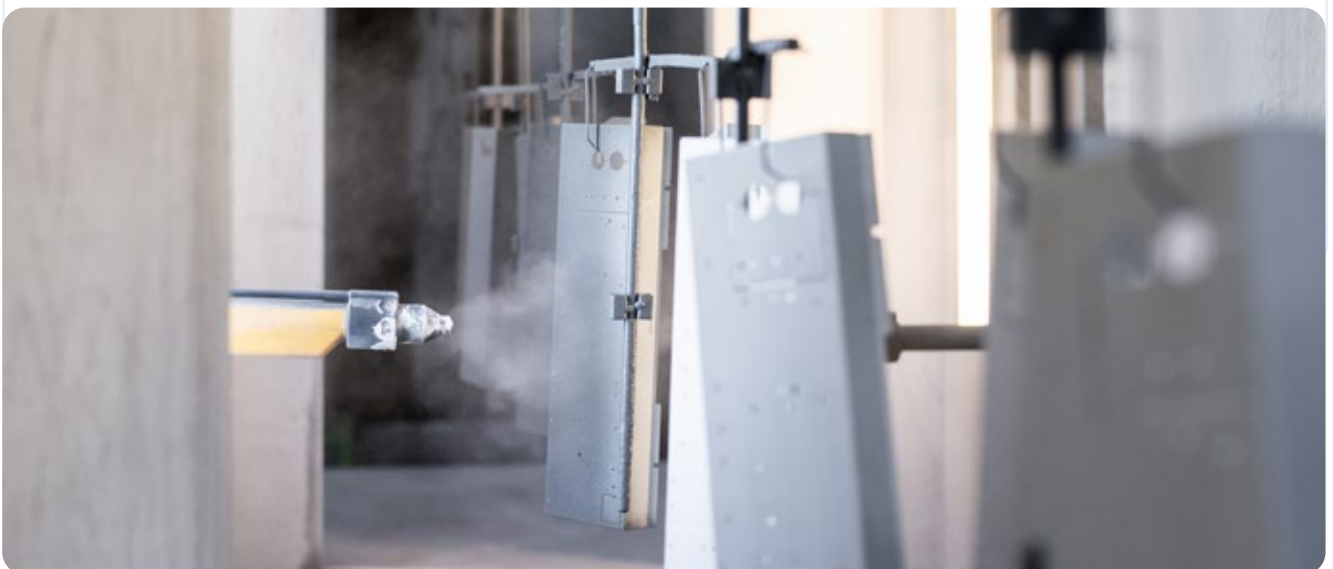
Thorlux powder coating facility utilising recycled powder
